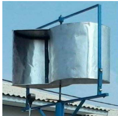
Gambar 3. Turbin Savonius h \neq 2D , D = 52 \text{ cm} , h = 36 \text{ cm}
