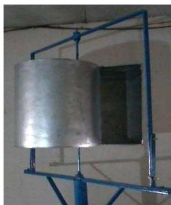
Gambar 2. Turbin Savonius h \neq 2D , D = 45 cm, h = 30 cm
